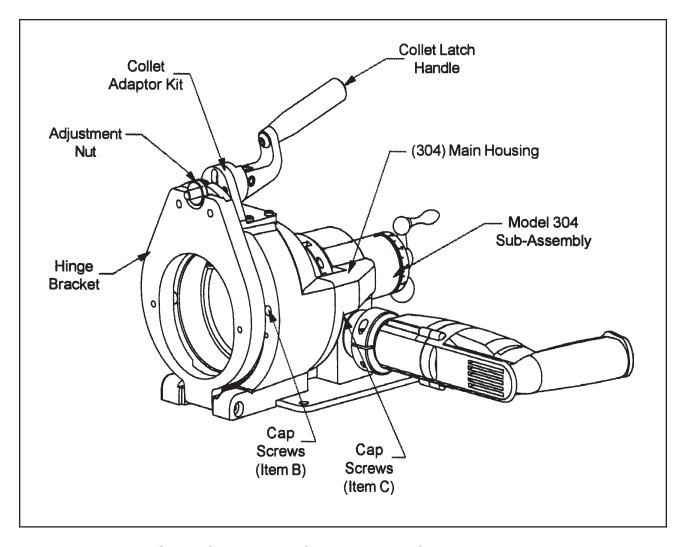
Remove the Collet, if there is one, from the inside of the Main Housing.
