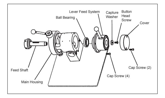
Remove the Button head screw and capture washer from the end of the feed shaft.
