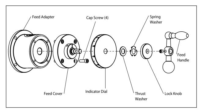
Remove the indicator dial from the feed shaft.
