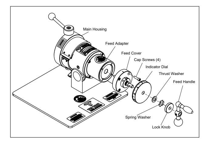
Rotate the feed cover so that the indicator mark is on the top.
