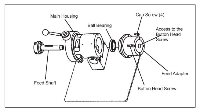
Slide the feed adapter onto the end of the main housing.
