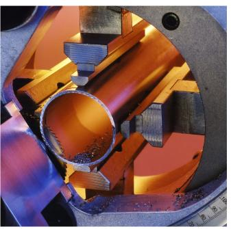
perfect tube to tube alignment with the smallest gap possible, removing the need to facing the tube therefore saving a significant amount of time and money.
